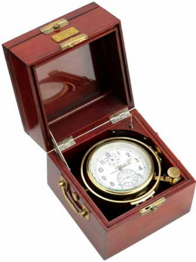
477 A MODERN RUSSIAN 56 HOUR MARINE CHRONOMETER XPOHOMETP MOPCKON TV 25-07 1533-84 The 4in. dial with Arabic numerals, single chain driven movement, the double case with brass gimbal and carrying handles, serial no. 18838 (with winder) 19cm wide, 19cm deep, 19.5cm high, (7in wide, 7in deep, 7 1/2in high) £400 - 600 €450 - 680
